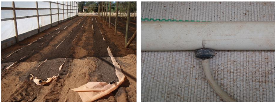
Figure 10 In-ground gutter system (left) and drippers and spaghetti tubing on secondary irrigation line (right)
